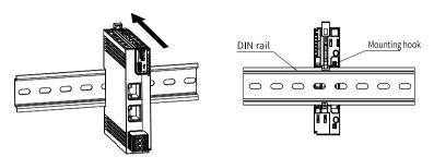
**Note:** After the module is installed, the DIN rail mounting hook will automatically move downward to lock the module to the rail. If the DIN rail mounting hook does not move downward, press down the top of it to ensure that the module is installed in place.
