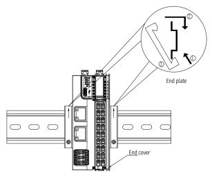
Install the end cover to the last module to prevent exposure of the metal pins. After installing the end cover, mount an end plate on either side of the module assembly to prevent sliding of the module.
